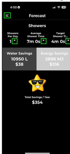
The calculation works by getting the time difference between the Average Shower Time and the Target Shower Time implemented by the ShowerStar device.
