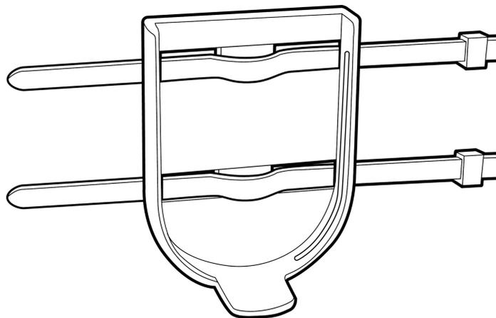
Wrap both cable ties around the pipe, then take the pointed end and insert it into the head of the cable tie, one at a time. Ratchet both cable ties tight to ensure the mounting cradle is properly fixed and does not slide along the shower pipes.
